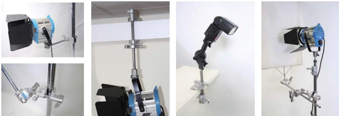
KCP-605, is 11.9" (30cm) long chain clamp with 6" (10" is also available for KCP-606) of steel chain. With the flexible chains, it can hold around any shape of wide size objects and adjust quickly by turning 5/8" baby stud in the rear of clamp. Meanwhile, the safety T-handle is also designed to eliminate any risks of unexpected looseness of the trigger.
